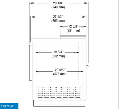
**IMPORTANT NOTE:** A minimum clearance of <u>3</u>" is required on each side, front and rear of cabinet for optimum performance.
