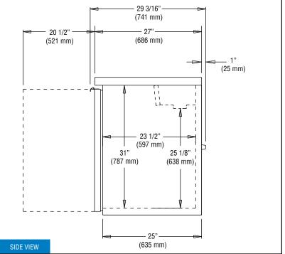
**IMPORTANT NOTE:** Models are completely front breathing and take in and exhaust air through the front
